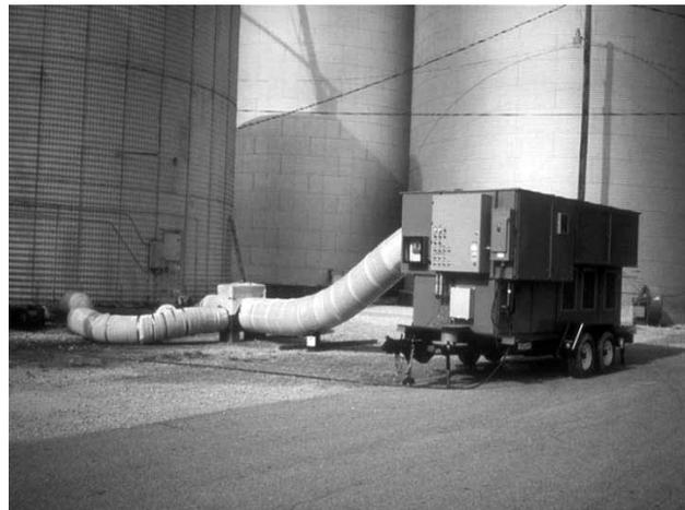
**Figure 1.** Grain chillers (from Burks et al. 2000).
