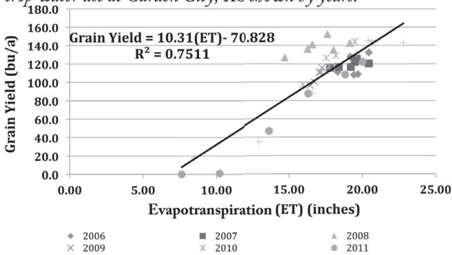
**Figure 3.** Yield response of grain sorghum at various levels of irrigation at Garden City, KS shown by years. Years 2006 – 2010 are near average or above precipitation (wet) years. 2011 – 2012 are drought (dry) years.
